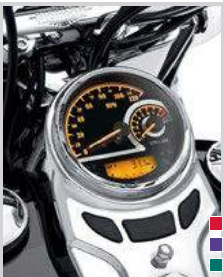
A. COMBINATION ANALOG SPEEDOMETER/TACHOMETER – 5" BLACK DIAL
